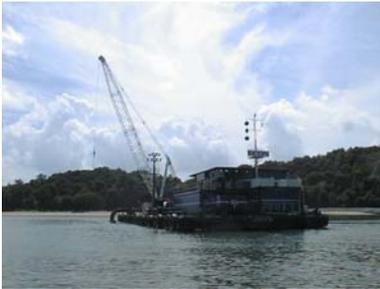
The contractor proposed to use three(3) splitter barges to transport the tetrapods and rocks offshore. Two(2) construction barges would be used with CCH1500E 150 tonne cranes to place the tetrapods and rock and for dredging works. An accuracy of 100mm was specified for position and depth monitoring during such work.
